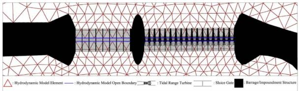
Arrangement of hydrodynamic model mesh (in plan view) around caissons, turbines and sluices for a tidal barrage or lagoon (from Angeloudis et al., 2016)
