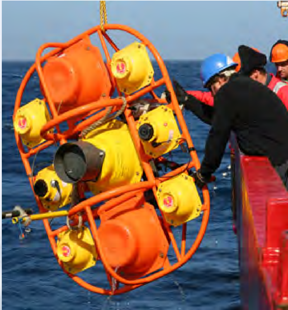
Deep-sea bottom pressure recorder of the National Oceanography Centre to measure the tide in depths of as much as 5000 m.
